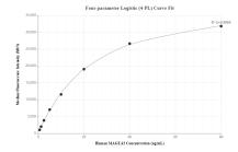
Cytometric bead array standard curve of MP00467-2, MAGEA3 Recombinant Matched Antibody Pair, PBS Only. Capture antibody: 83480-3-PBS. Detection antibody: 83480-4-PBS. Standard: Ag0265. Range: 0.625-80 ng/mL
