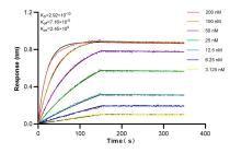
Biolayer interferometry (BLI) kinetic assays of 83375-2-RR against Mouse B7-H2/ICOSLG were performed. The affinity constant is 0.292 nM.
