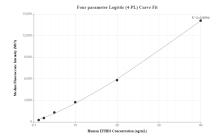
Cytometric bead array standard curve of MP00269-1, EFHD2 Recombinant Matched Antibody Pair, PBS Only. Capture antibody: 83264-1-PBS. Detection antibody: 83264-4-PBS. Standard: Ag35084. Range: 1.25-40 ng/mL
