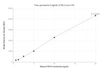
Cytometric bead array standard curve of MP00154-1, USP30 Recombinant Matched Antibody Pair, PBS Only. Capture antibody: 83240-2-PBS. Detection antibody: 83240-3-PBS. Standard: Ag7620. Range: 0.625-20 ng/mL 0.625-20 ng
