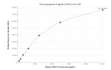
Cytometric bead array standard curve of MP00286-2, GPR35 Recombinant Matched Antibody Pair, PBS Only. Capture antibody: 83197-2-PBS. Detection antibody: 83197-4-PBS. Standard: SY01275. Range: 78.125-5000 pg/mL
