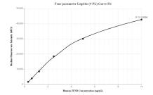
Cytometric bead array standard curve of MP00281-2, JUND Recombinant Matched Antibody Pair, PBS Only. Capture antibody: 83134-2-PBS. Detection antibody: 83134-3-PBS. Standard: SY00925. Range: 0.313-10 ng/mL
