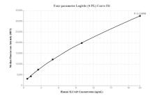
Cytometric bead array standard curve of MP00073-1, SLC 4A9 Recombinant Matched Antibody Pair, PBS Only. Capture antibody: 83076-2-PBS. Detection antibody: 83076-3-PBS. Standard: Ag34492. Range: 0.625-20 ng/mL.
