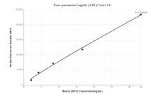
Cytometric bead array standard curve of MP00096-2, TRPS1 Recombinant Matched Antibody Pair - PBS only. Capture antibody: 83062-2-PBS. Detection antibody: 83062-1-PBS. Standard: Ag33959. Range: 1.25-20 ng/mL
