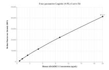
Cytometric bead array standard curve of MP00007-2, ADAMDEC 1 Recombinant Matched Antibody Pair, PBS Only. Capture antibody: 82985-5-PBS. Detection antibody: 82985-3-PBS. Standard:Ag12265. Range: 0.625-20 ng/mL
