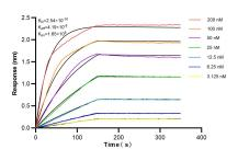
Biolayer interferometry (BLI) kinetic assays of 82983-2-RR against Human TMEM132E were performed. The affinity constant is 0.254 nM.
