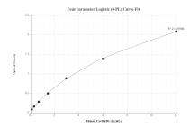
Sandwich ELISA standard curve of MP80003-1, Cyclin D1 Hybrid Matched Antibody Pair, PBS Only. Capture antibody: 68790-1-PBS. Detection antibody: 82681-1-PBS. Standard: Ag25384. Range: 0.188-12 ng/mL
