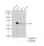
IP result of anti-ATG5 (IP:81803-1-RR, 4ug; Detection:81803-1-RR 1:2000) with HeLa cells lysate 1280 ug. This data was developed using the same antibody clone with 81803-1-PBS in a different storage buffer formulation.
