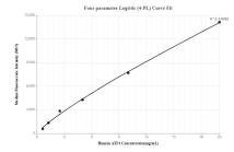
Cytometric bead array standard curve of MP00113-2, ATF 4 Recombinant Matched Antibody Pair, PBS Only. Capture antibody: 81798-3-PBS. Detection antibody: 81798-5-PBS. Standard: Ag1279. Range: 0.625-20 ng/mL
