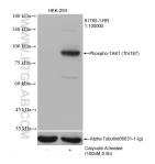
Non-treated and Calyculin A treated HEK-293 cells were subjected to SDS PAGE followed by western blot with 81785-1-RR (Phospho-TAK1 (Thr187) antibody) at dilution of 1:100000 incubated at room temperature for 1 hour. The membrane was stripped and re-blotted with Alpha Tubulin antibody as loading control.
