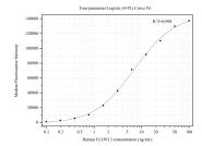
Cytometric bead array standard curve of MP50418-2, ELOVL3 Monoclonal Matched Antibody Pair, PBS Only. Capture antibody: 68964-3-PBS. Detection antibody: 68964-4-PBS. Standard:Ag24318. Range: 0.098-100 ng/mL
