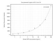
Cytometric bead array standard curve of MP50164-1, MPO Monoclonal Matched Antibody Pair, PBS Only. Capture antibody: 68797-1-PBS. Detection antibody: 68797-2-PBS. Standard:Eg0511. Range: 0.781-100 ng/mL
