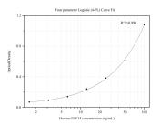
Sandwich ELISA standard curve of MP50133-3, GDF 15 Monoclonal Matched Antibody Pair, PBS Only. Capture antibody: 68768-3-PBS. Detection antibody: HRP-conjugated 68768-6-PBS. Standard:Ag33750. Range: 1.563-100 ng/mL
