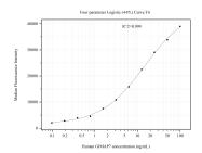
Cytometric bead array standard curve of MP50958-4, GIMAP7 Monoclonal Matched Antibody Pair, PBS Only. Capture antibody: 68451-1-PBS. Detection antibody: 68451-5-PBS. Standard:Ag10740. Range: 0.098-100 ng/mL
