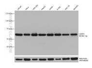
Various lysates were subjected to SDS PAGE followed by western blot with 68166-1-Ig (U2AF2 antibody) at dilution of 1:20000 incubated at room temperature for 1.5 hours. The membrane was stripped and reblotted with HRP-conjugated Beta Actin Monoclonal antibody (HRP-66009) as loading control.
