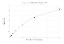
Sandwich ELISA standard curve of MP50054-1, IL11 Monoclonal Matched Antibody Pair - PBS only. 68135-2-PBS was coated to a plate as the capture antibody and incubated with serial dilutions of standard Ag11199. 68135-1-PBS was biotinylated as the detection antibody. Range: 6.25-400 pg/mL
