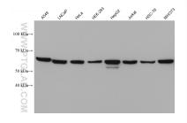
Various lysates were subjected to SDS PAGE followed by western blot with 68090-1-1g (FBXW11 antibody) at dilution of 1:5000 incubated at room temperature for 1.5 hours.
