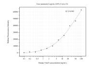
Cytometric bead array standard curve of MP50554-2, Tim23 Monoclonal Matched Antibody Pair, PBS Only. Capture antibody: 67535-3-PBS. Detection antibody: 67535-4-PBS. Standard:Ag27069. Range: 0.098-100 ng/mL.
