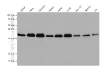
Various lysates were subjected to SDS PAGE followed by western blot with 67445-1-lg (HNRNPA2B1 antibody) at dilution of 1:20000 incubated at room temperature for 1.5 hours.
