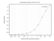
Sandwich ELISA standard curve of MP50209-1, MTOR Monoclonal Matched Antibody Pair, PBS Only. Capture antibody: 66888-2-PBS. Detection antibody: HRP-conjugated 66888-3-PBS. Standard:Ag28395. Range: 0.049-50 ng/mL
