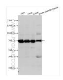
Various lysates were subjected to SDS PAGE followed by western blot with 66626-1-Ig (cIAP1 antibody) at dilution of 1:4000 incubated at room temperature for 1.5 hours.
