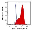
1X10^6 THP-1 cells were surface stained with 0.4 ug Anti-Human CD31 (66065-2-Ig, Clone:3F8E2) and CoraLite@488-Conjugated AffiniPure Goat Anti-Mouse IgG(H+L) at dilution 1:1000 (red), or 0.4 ug Control Antibody. Cells were not fixed.
