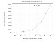
Cytometric bead array standard curve of MP51300-3, RAB4A Monoclonal Matched Antibody Pair, PBS Only. Capture antibody: 60886-4-PBS. Detection antibody: 60886-3-PBS. Standard:Ag20554. Range: 0.195-100 ng/mL
