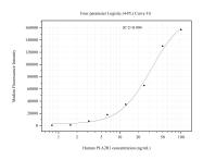
Cytometric bead array standard curve of MP51264-1, PLA2R1 Monoclonal Matched Antibody Pair, PBS Only. Capture antibody: 60853-1-PBS. Detection antibody: 60853-2-PBS. Standard:Ag22448. Range: 0.781-100 ng/mL
