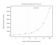
Cytometric bead array standard curve of MP51108-1, Claudin 5 Monoclonal Matched Antibody Pair, PBS Only. Capture antibody: 60779-1-PBS. Detection antibody: 60779-2-PBS. Standard:Ag33875. Range: 1.563-100 ng/mL
