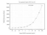
Cytometric bead array standard curve of MP51072-1, WDR78 Monoclonal Matched Antibody Pair, PBS Only. Capture antibody: 60742-1-PBS. Detection antibody: 60742-2-PBS. Standard:Ag27018. Range: 0.098-100 ng/mL.
