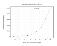
Cytometric bead array standard curve of MP50976-2, Presenilin-1 Monoclonal Matched Antibody Pair, PBS Only. Capture antibody: 60678-3-PBS. Detection antibody: 60678-4-PBS. Standard:Ag14464. Range: 0.391-100 ng/mL
