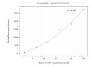
Cytometric bead array standard curve of MP50522-1, VAMP7 Monoclonal Matched Antibody Pair, PBS Only. Capture antibody: 60411-1-PBS. Detection antibody: 60411-2-PBS. Standard:Ag36541. Range: 3.125-100 ng/mL
