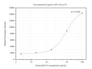
Sandwich ELISA standard curve of MP50002-1, KRT15 Monoclonal Matched Antibody Pair, PBS Only. Capture antibody: 60247-1-PBS. Detection antibody: HRP-conjugated 60247-2-PBS. Standard: Ag0185. Range: 0.313-20 ng/mL Cytometric bead array standard curve of MP50002-1, KRT 15 Monoclonal Matched Antibody Pair, PBS Only. Capture antibody: 60247-1-PBS. Detection antibody: 60247-2-PBS. Standard: Ag0185. Range: 1.563-100 ng/mL
