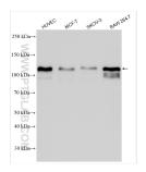
Various lysates were subjected to SDS PAGE followed by western blot with 29948-1-AP (ADAM17 antibody) at dilution of 1:8000 incubated at room temperature for 1.5 hours.
