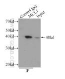
IP result of anti-MCL1 (IP:16225-1-AP, 3ug; Detection:16225-1-AP 1:1000) with Raji cells lysate 800ug.
