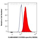
1X10^6 U-937 cells were intracellularly stained with 0.8 ug CoraLite® Plus 488 Anti-Human CXCR3B-specific (CL488-60065, Clone:1B2D6) (red), or 0.8 ug Mouse IgC2b Isotype Control (CL488-66360-3, Clone: K11B8C4B5) (blue). Cells were fixed with 4% PFA and permeabilized with Flow Cytometry Perm Buffer (PF00011-C).
